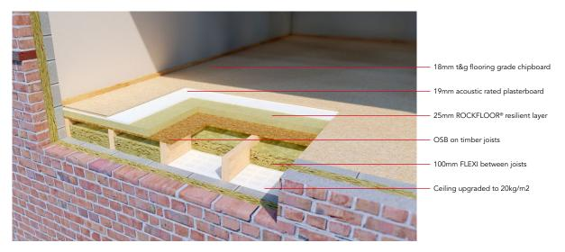
Note: If the existing ceiling is being replaced the sound performance of the floor can be further enhanced by fitting resilient bars which isolate the ceiling from the floor structure.
